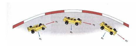
• When acceleration and velocity are perpendicular to each other, turning occurs.
