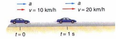
• When acceleration and velocity are in the same direction, speed increases.
