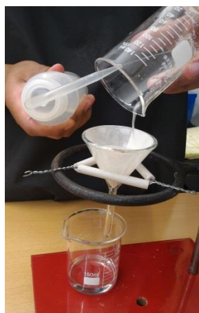
Figure 5. How to remove the solid sample using a wash bottle.
