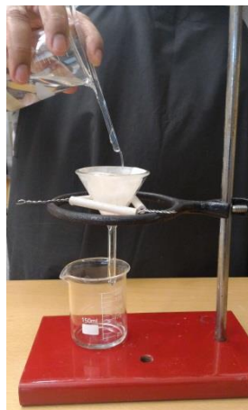
Figure 4. Proper technique for pouring a mixture using a beaker.
