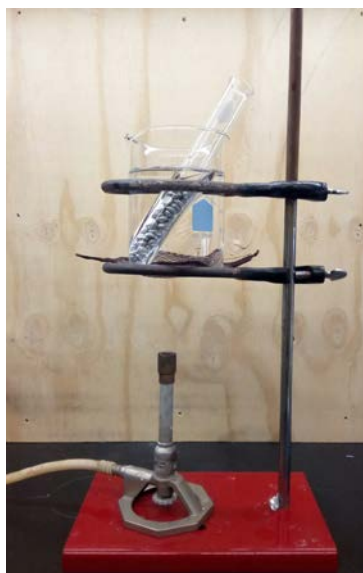
Figure 2. Water bath set up with unknown sample.
