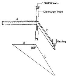
You will work in pairs and record the positions of the helium spectral lines on the spectroscope scale (meter stick "a"). You will use these data to prepare a "calibration curve" by plotting the measured positions against the known wavelengths of the lines, which are:
